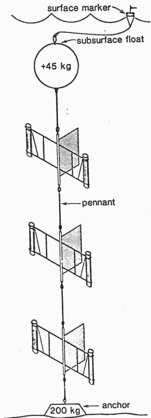
Figure 4. Schematic diagram of sediment trap used in VFX monitoring.
