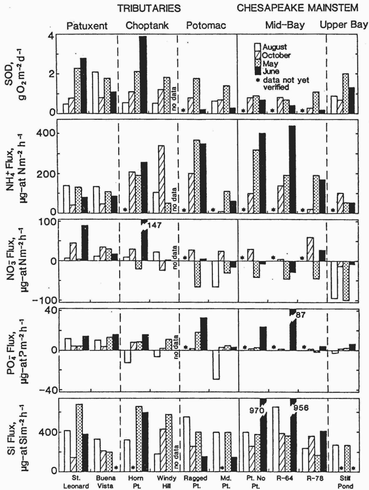
Fig. 5. Average sediment-water exchanges of oxygen (SOD), ammonium ( $\text{NH}_4^+$ ), nitrate ( $\text{NO}_3^-$ ), dissolved inorganic phosphorous ( $\text{PO}_4^{2-}$ ) and silicic acid (Si) at SONE stations for the period August, 1984-June, 1985. Negative values for nutrient fluxes indicate fluxes from water to sediments. All SOD fluxes were from water to sediments. Asterisks indicate data not yet verified.
