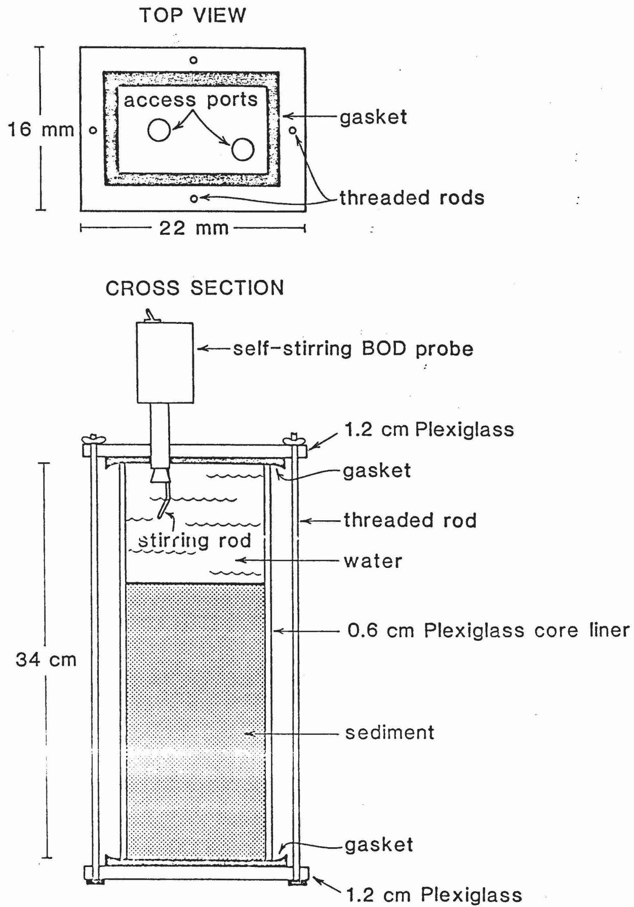
Figure 3. Schematic diagram of the incubation chamber used in the SONE program.
