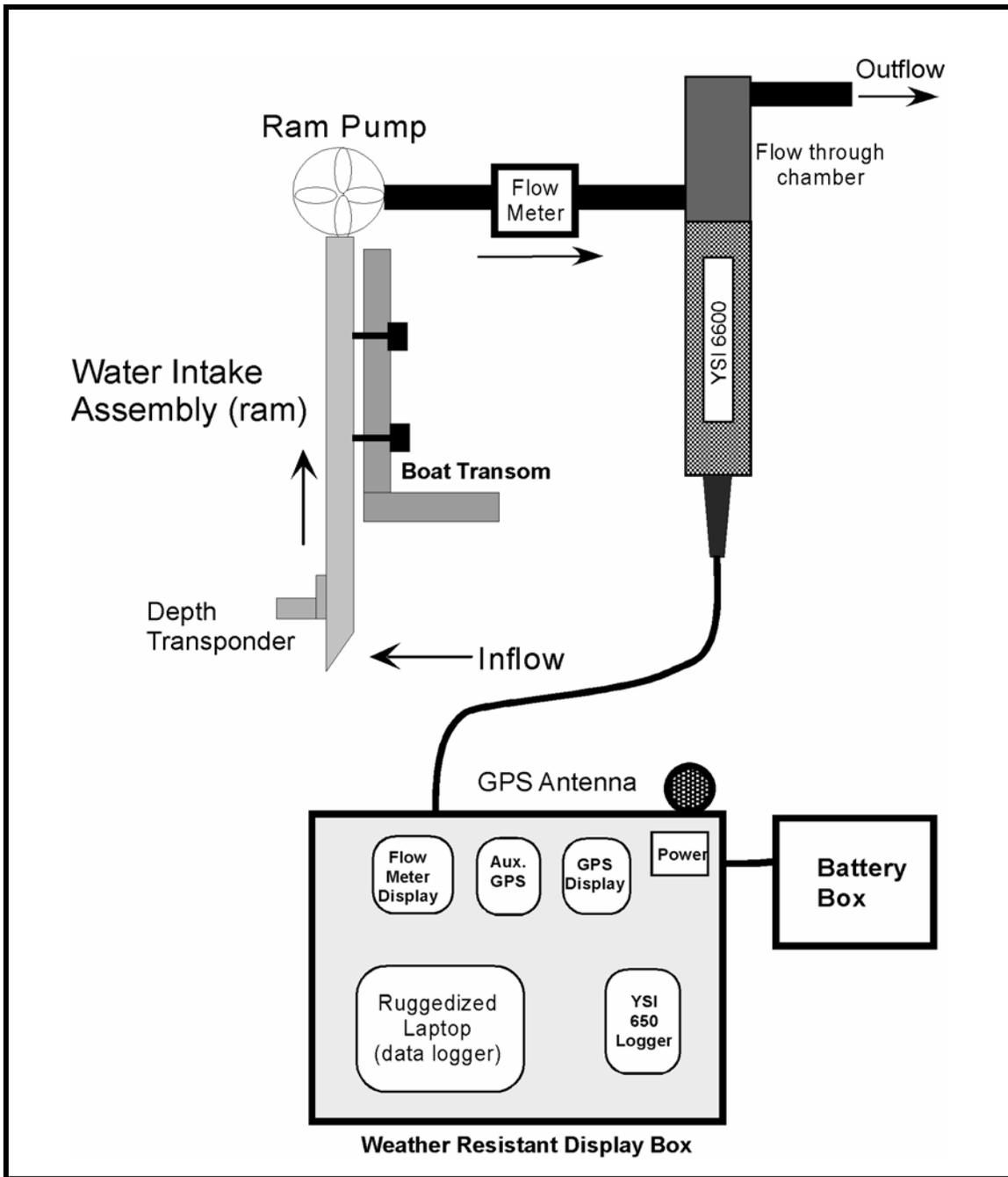
**Figure 3-1.** Schematic diagram of Dataflow 5.5 illustrating the path of water through the instrument.
