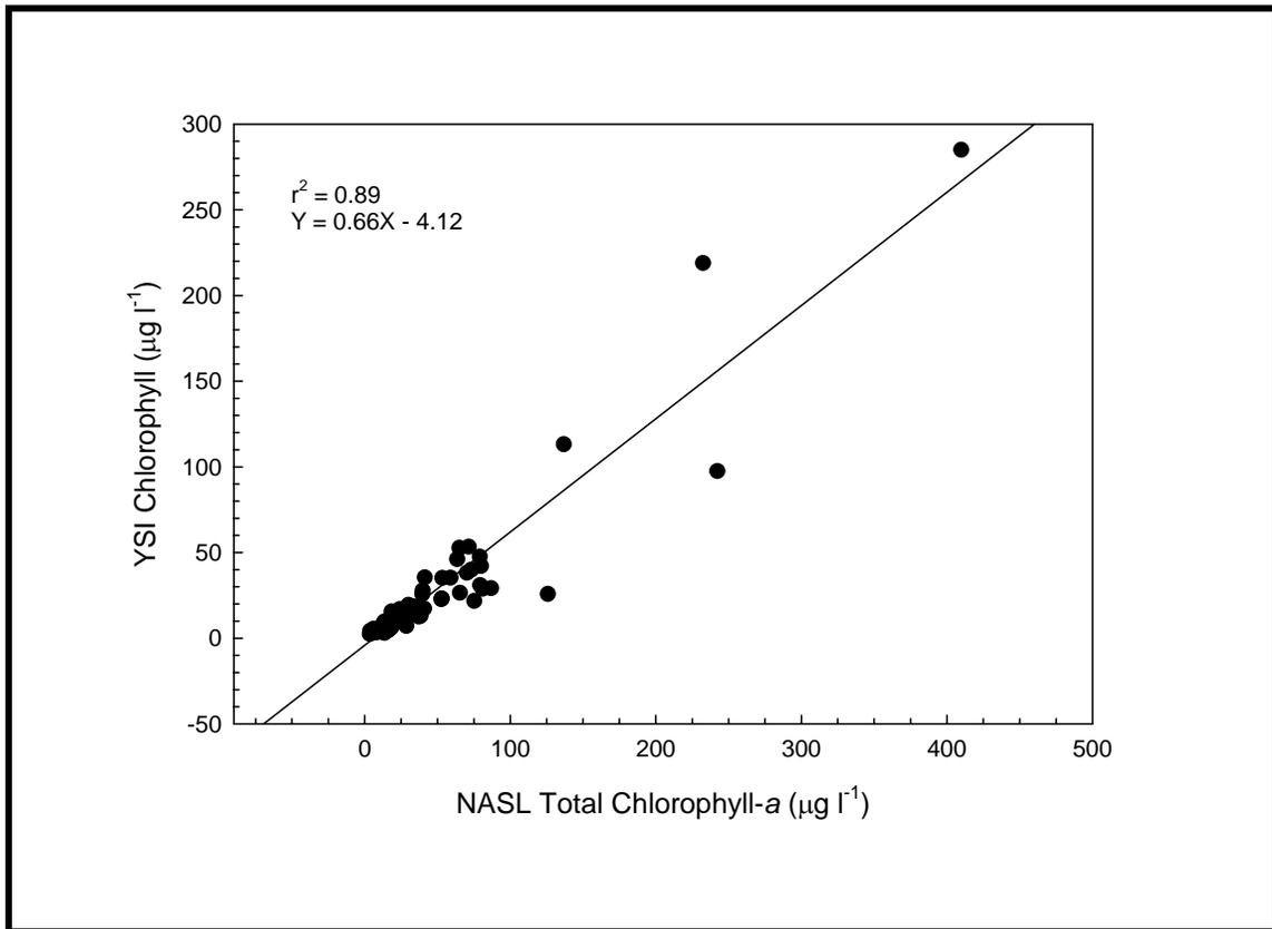
**Figure 3-13.** Correlation between laboratory extracted total chlorophyll-*a* and YSI datasonde chlorophyll concentrations on the Patuxent River estuary, 2003.
