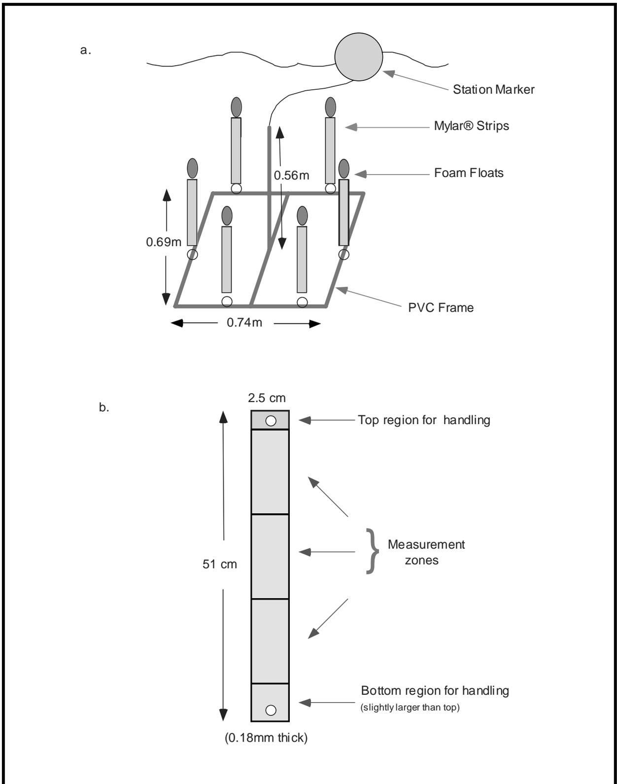
**Figure 4-2.** Diagram of a) epiphyte collector array and b), individual Mylar® strip.
