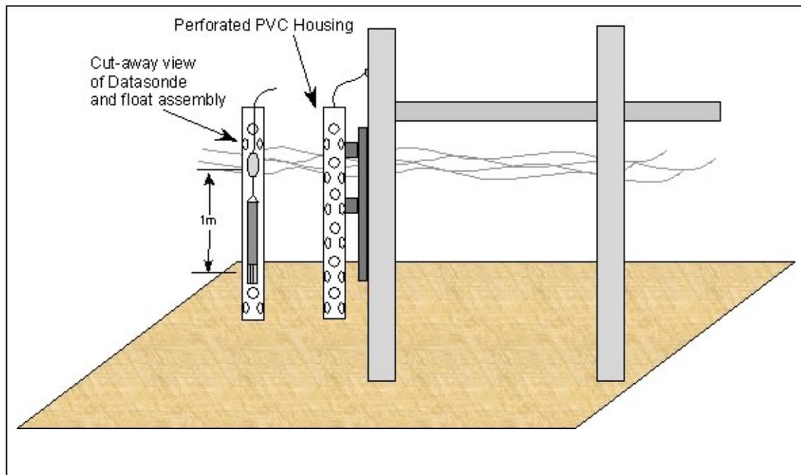
**Figure 2-2.** Diagrammatic sketch of the continuous monitoring setup in 2003 at stations located at CBL, Benedict, and Kings Landing. The configuration at Pin Oak was similar, except the datasonde was fixed off the bottom and did not float with the tide as pictured above.
