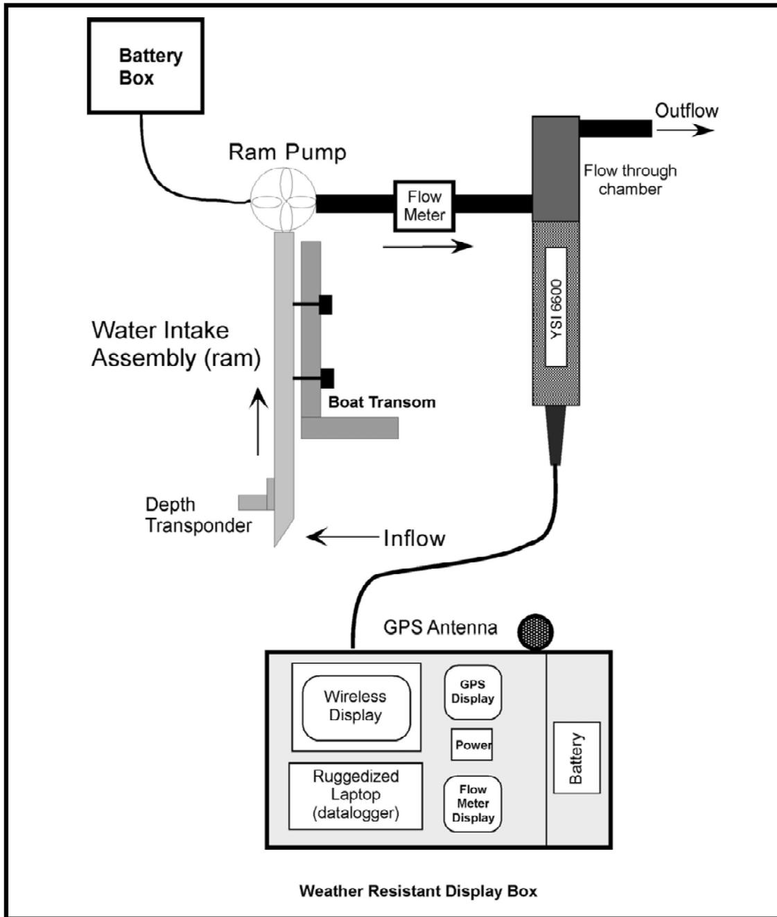
Figure 2.2-1. Schematic diagram of DATAFLOW© illustrating the path of water through the instrument.
