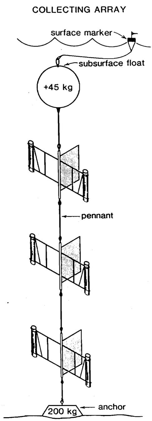
Fig. 3-4. Schematic diagram of the sediment trap used in VFX monitoring.
