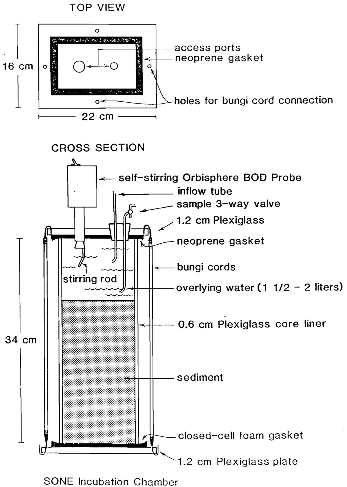
Fig. 3-3. Schematic diagram of the incubation chamber used in SONE program.
